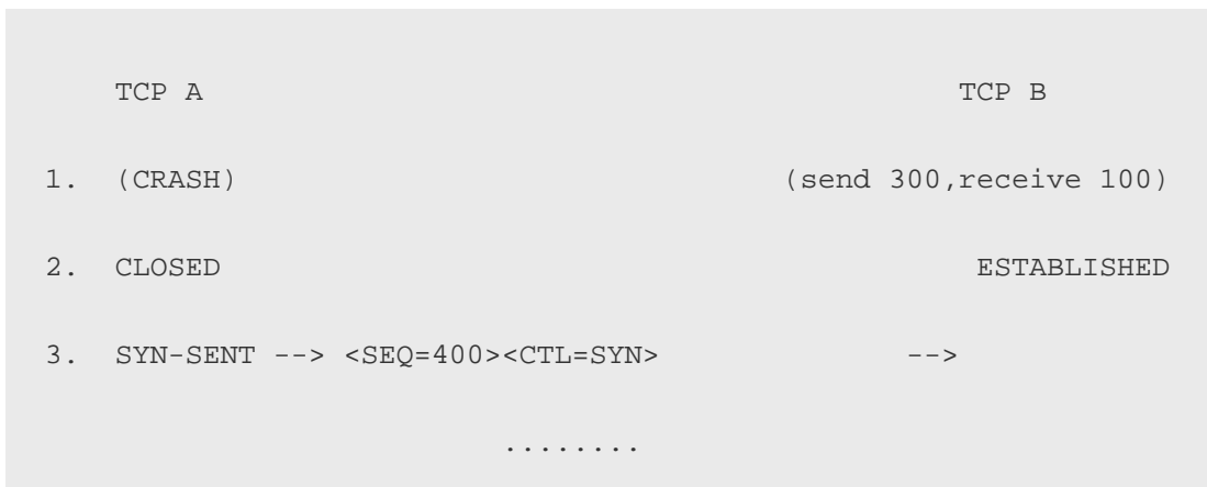
Figure 18: Half-Open Connection Discovery with the proposed counter-measure
