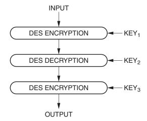
During encryption, the input is first encrypted with the first key, then decrypted with the second key and finally encrypted with the third key. During decryption, the key sequence and encryption/decryption block sequence is reversed, as illustrated in Figure 4.
