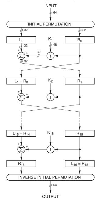
Figure 2 illustrates how a single block of data is being encrypted. First, the order of the input bits is changed according to the permutation function. The low 32 bits  $(R_0)$  are then processed separately from the high 32 bits  $(L_0)$ . There are 16 process steps, each step
