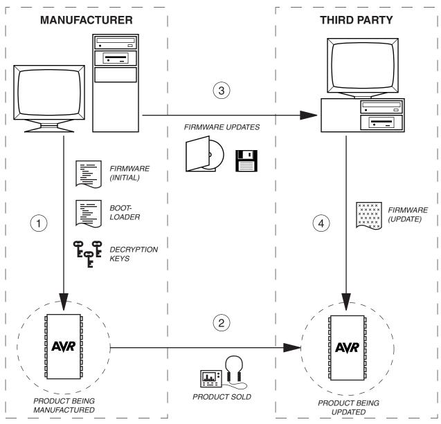
Notes: 1. During manufacturing, the microcontroller is first equipped with bootloader, decryption keys and application firmware. The bootloader takes care of receiving the actual
