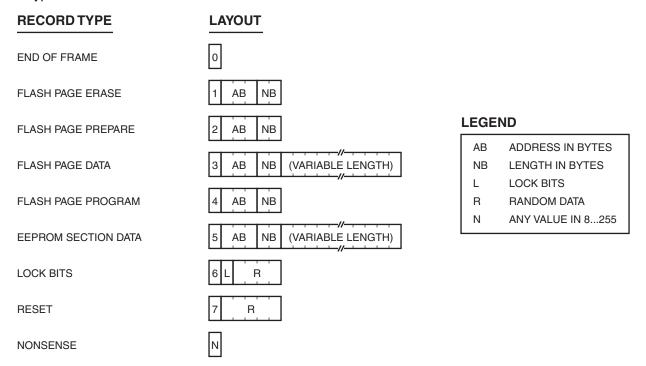
The record type is given as the first byte in the record. The application data is broken down to record types 1, 2, 3 and 4 (i.e., erase, prepare, load and write buffer page to Flash). The data for the EEPROM section is formatted into record type 5. Lock bits are sent in record type 6. Record types 0 and 7 are for ending a frame and transmission, respectively.
