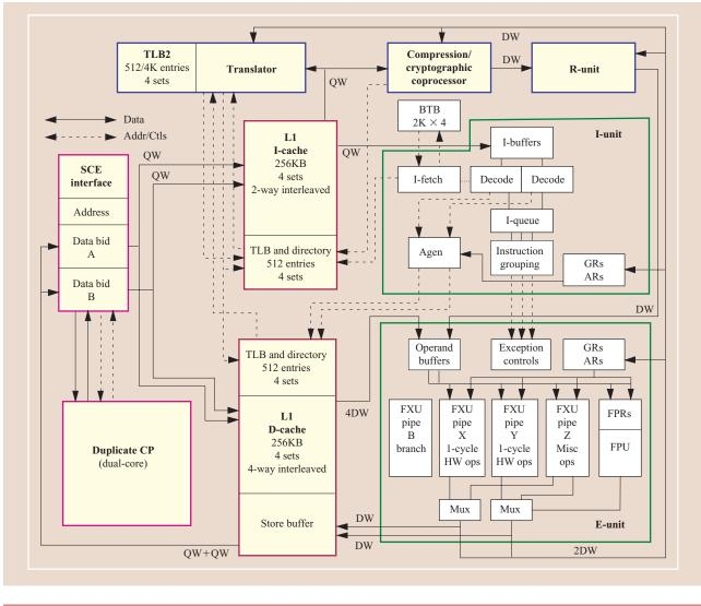
Diagram of z990 processor. (DW: doubleword; QW: quadword; ARs: access registers; FPRs: floating-point registers; HW ops: hardware executed instructions.)
