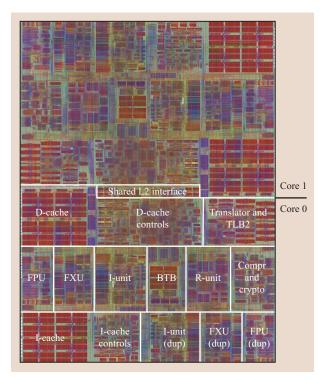
Micrograph of z990 processor chip.
