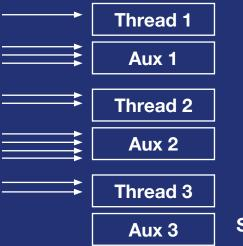
Each worker thread has an auxiliary thread Worker thread uses "poll()" Auxiliary thread uses "epoll()" Worker thread passes idle connections to auxiliary thread When a connections becomes active auxiliary thread passes connection to the worker thread
