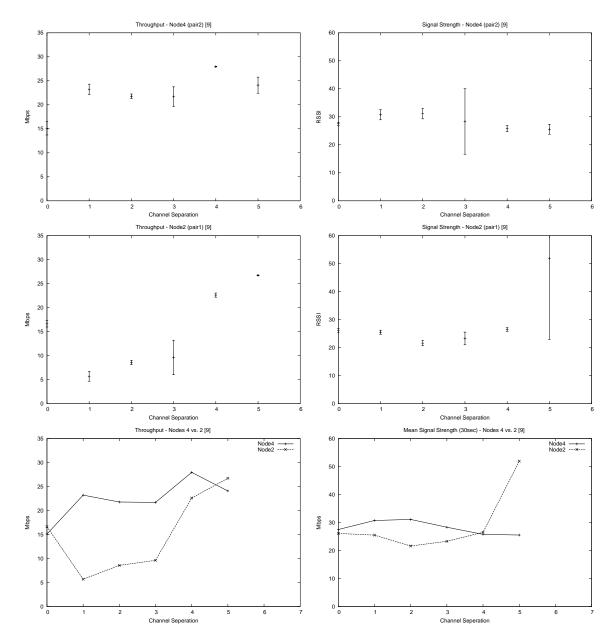
Figure 8: Signal and throughput measurements from each network, and overlapping comparisons. Polarization has a significant effect when operation on the same channel.
