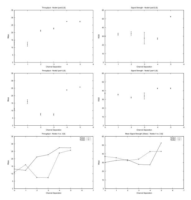
Figure 4: Signal and throughput measurements from each network, and overlapping comparisons. Noticeable improvements in performaces vs.  $90^{\circ}$  and  $180^{\circ}$
