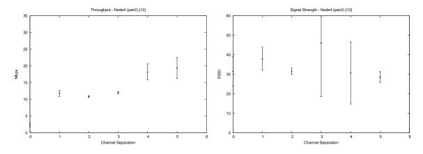
Figure 11: Signal and throughput measurements, interference from cars
