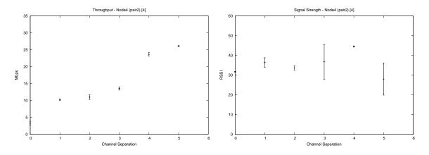
Figure 3: Signal and throughput measurements, throughput increases steadily but is poor on channel 1
