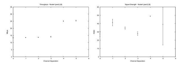
Figure 5: Signal and throughput measurements, much better performance on channel 1. Routing enforces better sharing of bandwidth
