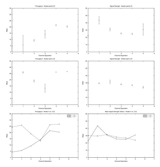
Figure 6: Signal and throughput measurements from each network, and overlapping comparisons.  $90^{\circ}$  configuration, pair1 network is dominating the available bandwidth on contended channels
