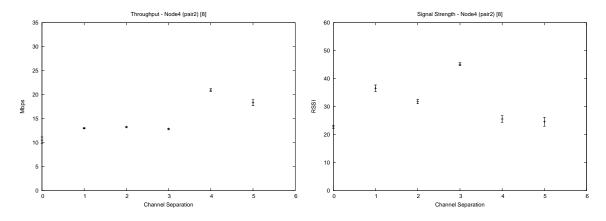
Figure 7: Signal and throughput measurements, 90  $^\circ$  configuration with routing.
