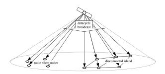
Figure 6. Broadcast and datacycle to silent nodes
