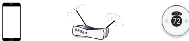
1008 Figure 4 illustrates an example of the Roles in a scenario where a smart phone sends a request 1009 message to a thermostat; the original request is sent over HTTP, but is translated into a CoAP 1010 request message by a gateway in between, and then delivered to the thermostat. In this 1011 example, the smart phone takes the role of a Client, the gateway takes the role of an 1012 Intermediary and the thermostat takes the role of a Server.
