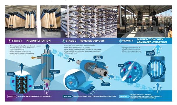
**Fig. 7.** Advanced water treatment process at the Water Replenishment District of Southern California (WRD) Leo J. Vander Lans Water (LVL) Treatment Facility [57]. Stage 3 includes the use of UV radiation for the disinfection of microorganisms and other components that are broken down due to advanced oxidation processes catalyzed by photolysis reactions of water with UV radiation. Figure credit: WRD LVL.
