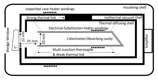
Fig. 1. A cross section of the C4 instrument.
