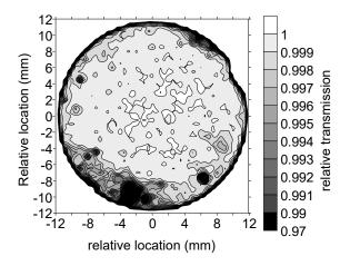
Fig. 6. Spatial transmissivity of the legacy C4-1 window normalized to the transmissivity at the geometric center of the window.
