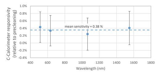
Fig. 4. Relative responsivity of the calorimeter after cleaning when compared to precleaning responsivity. Error bars are at k = 2.
