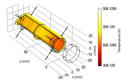
**Fig. 9.** C-calorimeter's steady-state heat map when no electrical or laser power is applied. Thermopiles are depicted by radial lines. The placement of this cavity and window within the instrument vacuum enclosure is depicted in Fig. 1. The unshaded element 20 mm in front of the cavity entrance depicts the fused silica wedged vacuum window.
