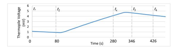
Fig. 2. Thermopile voltage for the C4 calorimeter during a typical measurement sequence with approximately 110 mW injected for 200 s starting at t = 80 s.
