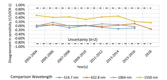
Fig. 3. Disagreement in sensitivity of the C4 instruments compared to NIST's LOCR.
