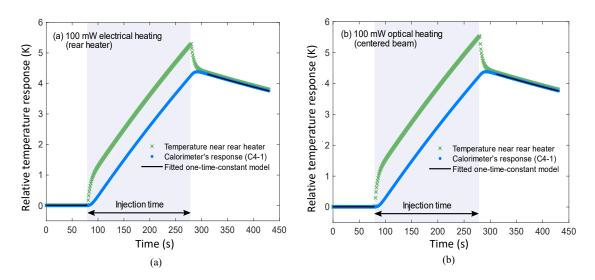
Fig. 10. Time-dependent response of C-calorimeter C4-1 to electrical heating (a) and optical heating (b) plotted as blue circles. The absorber near the heater (green crosses) heats and cools faster than the outermost surface of the cavity structure. The one-time-constant model in Eq. (1), presented as black lines, was fitted to the calorimeter's response.
