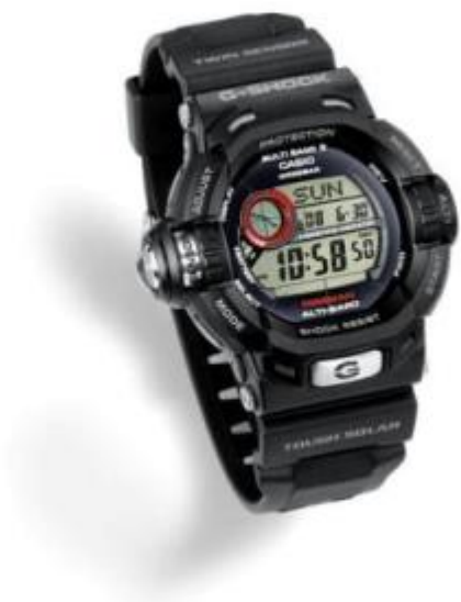
Fig. 23. A Casio “Multi Band 6” wristwatch. Introduced in 2008, these devices can synchronize to LF time signals from China (68.5 kHz), Germany (77.5 kHz), Japan (40 and 60 kHz), and the United Kingdom (60 kHz), in addition to the 60 kHz signal from WWVB (courtesy of Casio).
