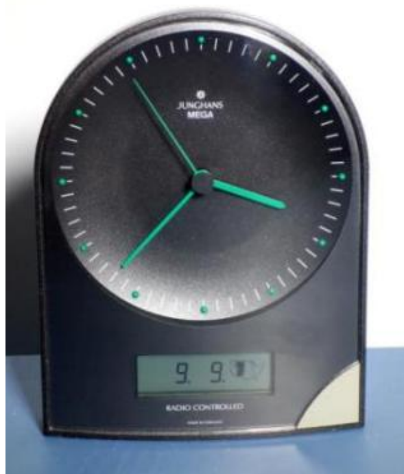
Fig. 22. The Junghans MEGA, introduced in the United States around 1996, was probably the first low cost WWVB radio controlled clock (A. Novick, NIST).
