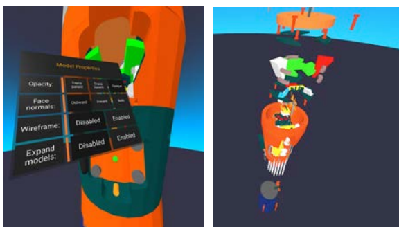
Figure 60. Left: STM with menu on the VR controller. Right: Exploded parts view of the STM.
