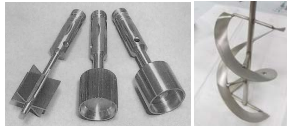
Figure 7. Rheometer spindles. The rotational speed of the spindle with a given applied torque can be used to infer viscosity. Left: traditional blade designs. Right: a novel helical design.
