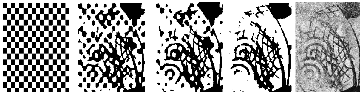
Figure 35. Segmentation of the shoeprint in a crime scene image (rightmost) obtained by the phase field function evolution (left 1-4) of a checkerboard initialization.
