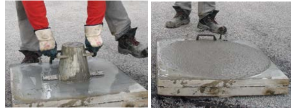
Figure 6. The slump flow test to assess flowability and flow rate, state-of-the-art since 1918. Left: lifting the cement-filled cone. Right: diameter of the resulting flow is measured. [Images: Wikimedia Commons author Knipptang, CC BY-SA 4.0]
