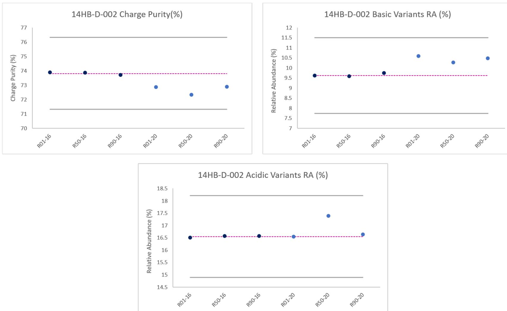
**Figure 16.** Charge heterogeneity control charts using capillary zone electrophoresis for lot 14HB-D-002. Initial certification (0y) data is shown in dark blue and 5YSV (5y) in light blue. Pink dotted line corresponds to the non-certified value assigned in the original 2016 certification. Control limits set at  $\pm 3u_c$  (grey bars)
