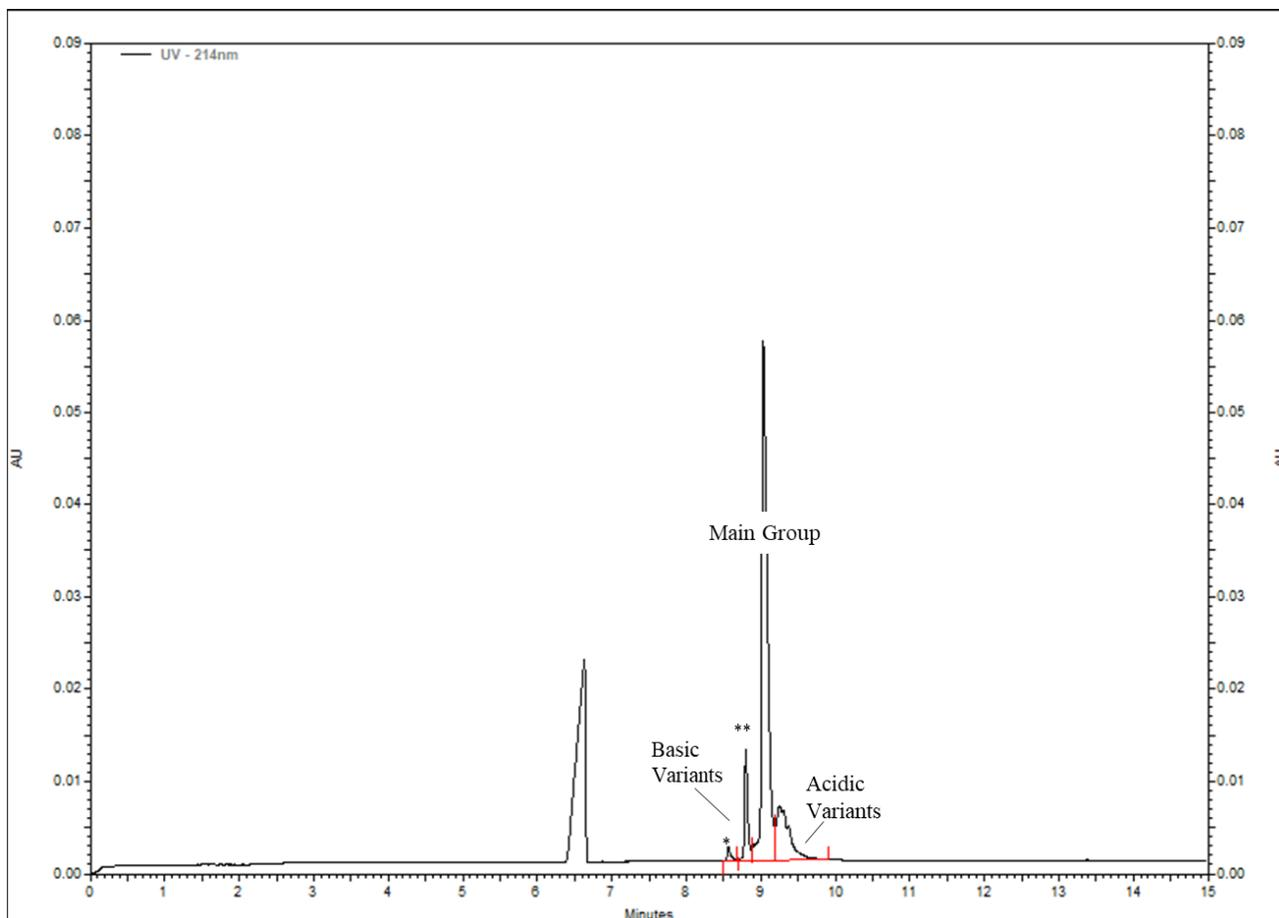
**Figure 14.** Representative electropherogram for lot 14HB-D-002 by CZE. Baseline and integration limits are indicated by red horizontal and vertical lines, respectively. (\*) indicates 1K (1 des-lysine) peak. (\*\*) indicates 2K (0 des-lysine) peak.
