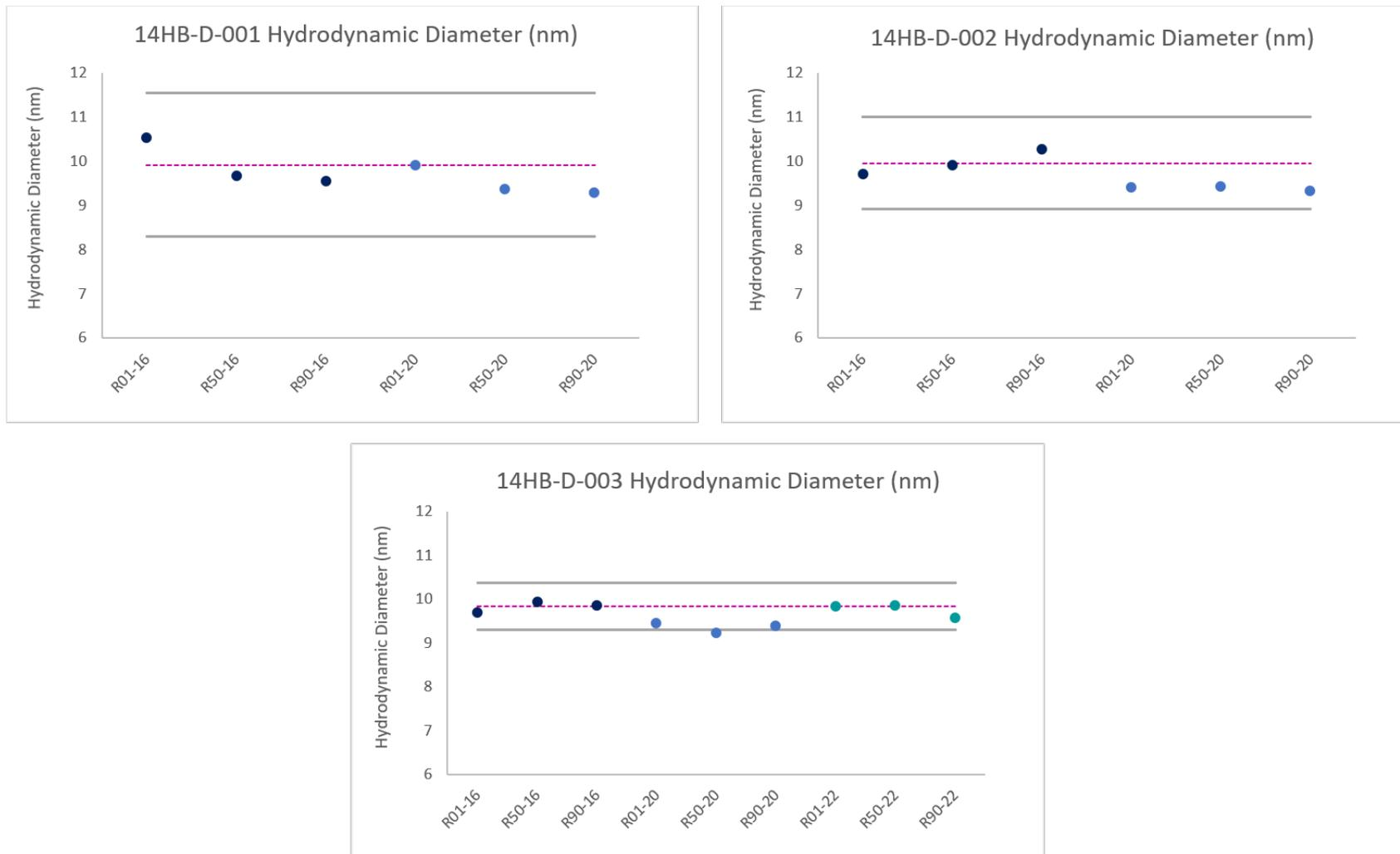
**Figure 19.** Average hydrodynamic diameter control charts using dynamic light scattering for lots 14HB-D-001, 14HB-D-002, and 14HB-D-003. Initial certification (0y) data is shown in dark blue, 5YSV 2020 (5yA) in light blue, 5YSV 2022 (5yB) in green. Pink dotted line corresponds to the non-certified value assigned in the original 2016 certification. Control limits set at  $\pm 3u_c$  (grey bars)
