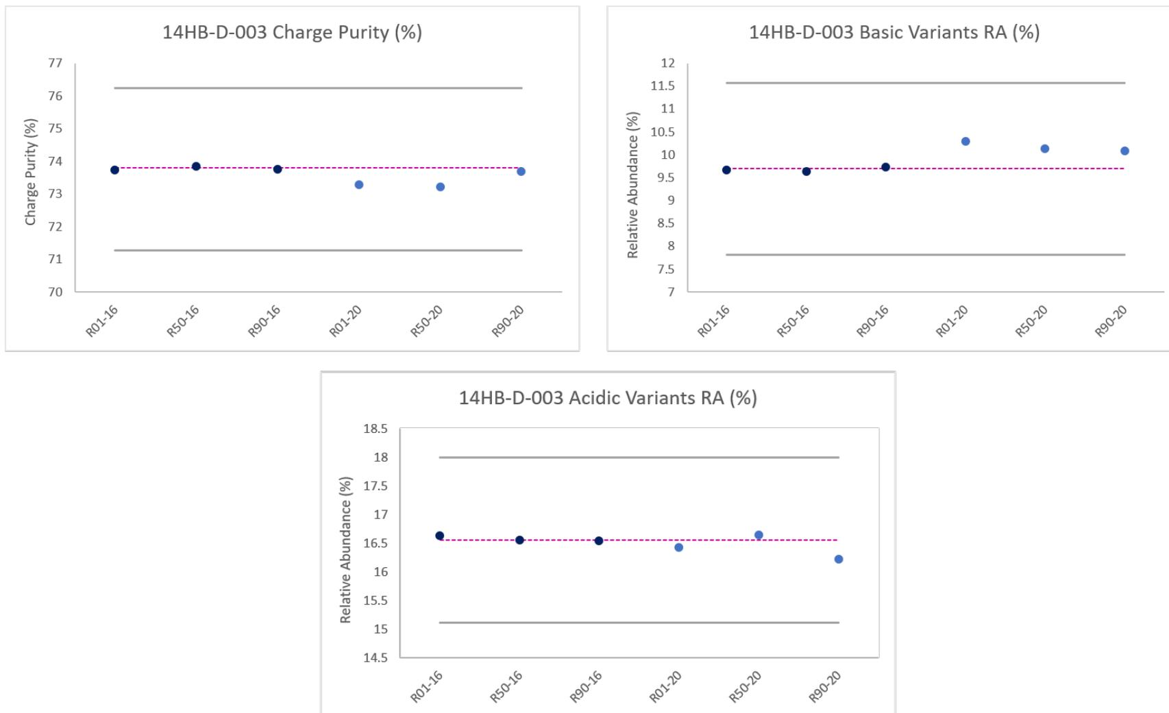
**Figure 17.** Charge heterogeneity control charts using capillary zone electrophoresis for lot 14HB-D-003. Initial certification (0y) data is shown in dark blue and 5YSV (5y) in light blue. Pink dotted line corresponds to the non-certified value assigned in the original 2016 certification. Control limits set at  $\pm 3\sigma_c$  (grey bars).
