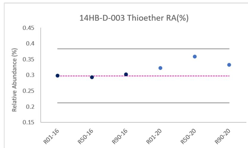
**Figure 13.** Size Heterogeneity control charts using capillary electrophoresis for lot 14HB-D-003. Initial certification (0y) data is shown in dark blue and 5YSV (5y) in light blue. Pink dotted line corresponds to the non-certified value assigned in the original 2016 certification. Control limits set at  $\pm 3u_c$  (grey bars)
