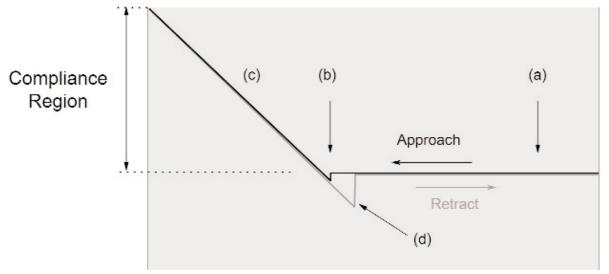
Fig. D 3 Example of AFM approach-retract curves.
