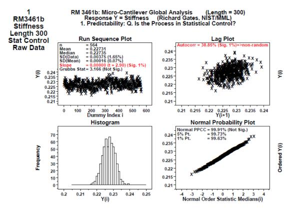
Fig. B 1 Global (n=564) stiffness statistical control example for 300 μm long cantilevers. and also for just the mean stiffness data (n=94),
