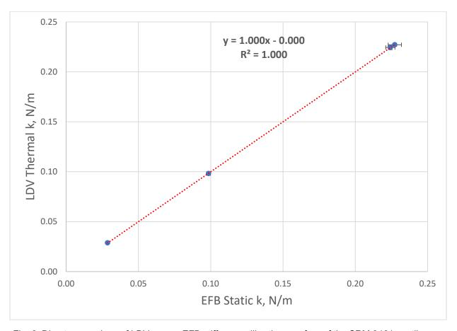
Fig. 6 Direct comparison of LDV versus EFB stiffness calibrations on four of the SRM 3461 cantilevers.
