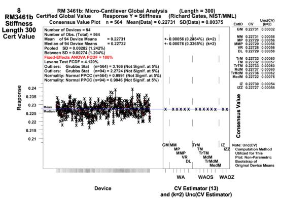
Fig. B 3 Global mean (GM) stiffness consensus value (n=94) example for 300 µm long cantilevers.
