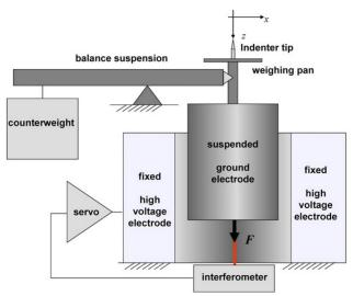
Fig. C 1 Electrostatic Force Balance Schematic, after [14].
