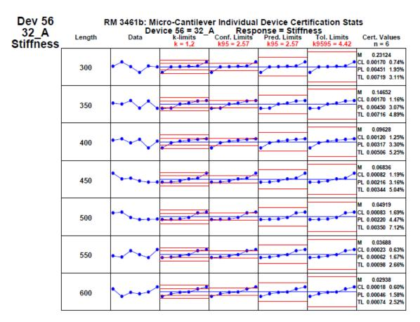
Fig. B 4 Individual device stiffness certification example (n=6) for device 32 A.
