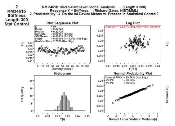
Fig. B 2 Global mean (n=94) stiffness statistical control example for 300 μm long cantilevers. as well as consensus value plots for all devices:
