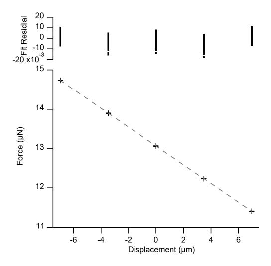
Fig. C 2 Force vs. displacement and linear fit residuals from the EFB test of the reference cantilever array W 23 D, 300 um long cantilever. Note, the slope of the fitted line (and determined stiffness) is negative because of the sign convention chosen for the force and displacement.
