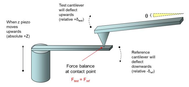
Fig. D 2 Schematic for contact between test and reference cantilevers.
