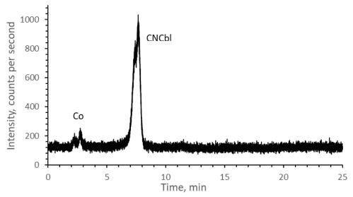
Figure 16. Exemplar LC-ICP-MS Chromatogram for Cyanocobalamin in SRM 3289.
