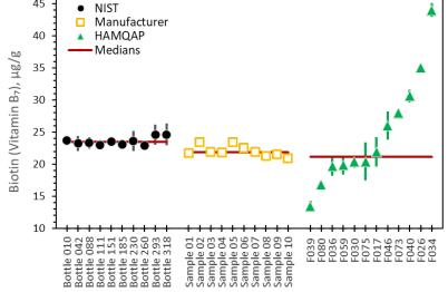
Figure 28. Measurement Results for Biotin (Vitamin B<sub>7</sub>),  $\mu g/g$  Symbols represent mean values; error bars represent one standard deviation.
