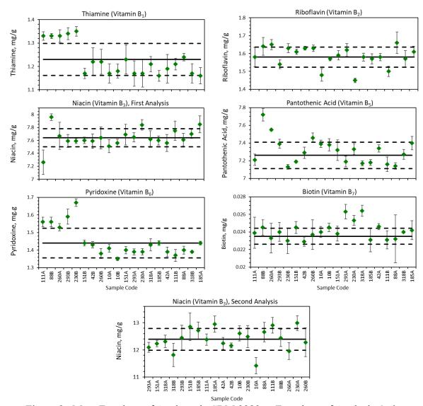
Figure 8. Mass Fractions of Analytes in SRM 3289 as Functions of Analysis Order Green diamonds represent results of the analysis of one of the two SRM 3289 preparations from each bottle. Solid lines denote the mean value; dashed lines bound one standard deviation (SD) above and below the mean. Error bars represent the SD for the three transitions averaged to determine the value.
