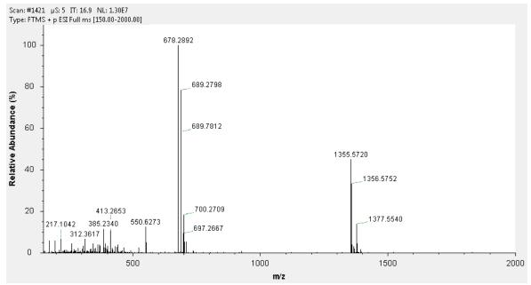
Figure 18. HR-MS Spectrum of the Cyanocobalamin Standard
