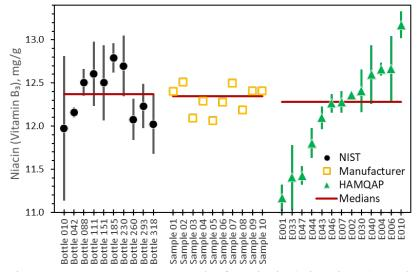
Figure 25. Measurement Results for Niacin (Vitamin B<sub>3</sub>), mg/g Symbols represent mean values; error bars represent one standard deviation.
