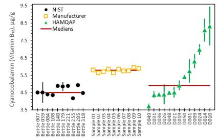
Figure 30. Measurement Results for Cyanocobalamin (Vitamin B<sub>12</sub>), µg/g Symbols represent mean values; error bars represent one standard deviation.
