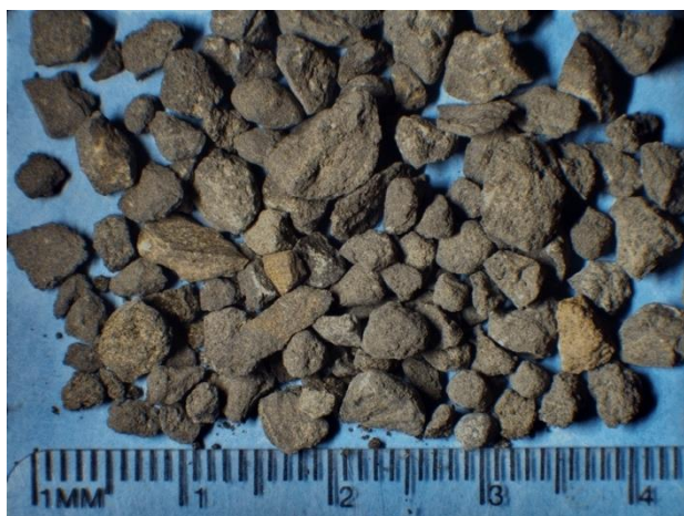
Figure 1 Crushed and sieved clinker fragments range in size between 2 mm and 5 mm.
