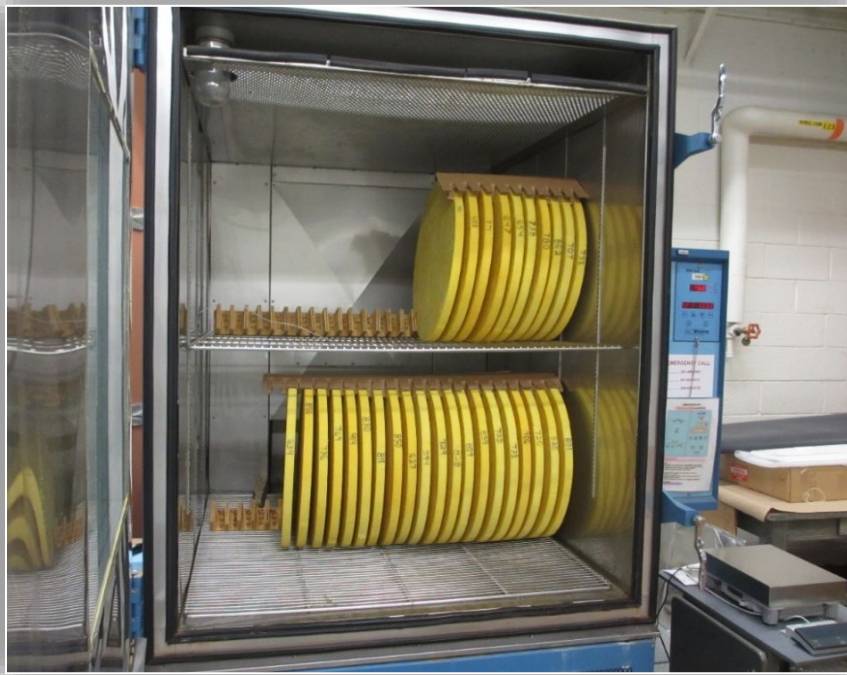
Fig. 13. Test specimens (500 mm diameter) in a large conditioning chamber.
