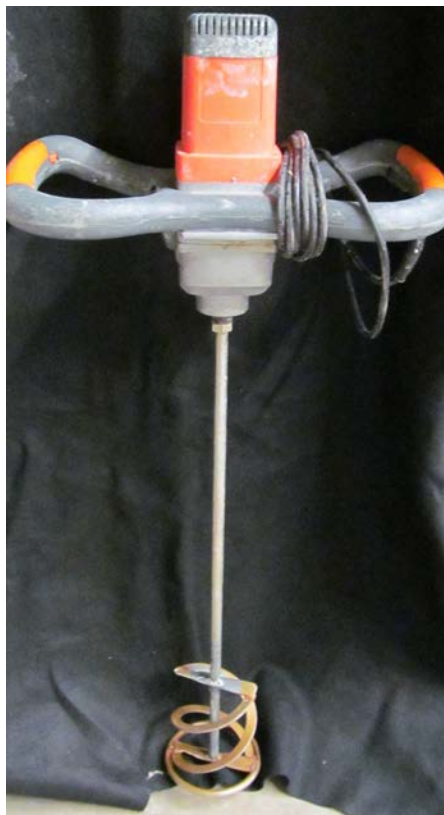
Figure 4: Picture of the impeller of hand-held mixer used for mixing the materials.
