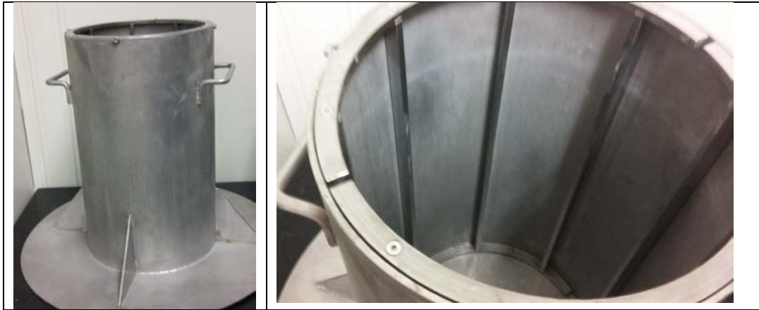
Figure 9: Container for the concrete measurements
