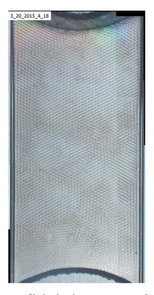
Figure 1: Emergence of lattice domain structure across a microfluidic plate. Channel dimensions ( $L\times W\times H$ ) of the Ibidi #80621  $\mu$ -Slide VI-flat hydrophobic are nominally 17 mm  $\times$  3.8 mm  $\times$  400  $\mu$ m. The mean diameter of the self-assembled aqueous emulsion droplets is on the order of 100  $\mu$ m.
