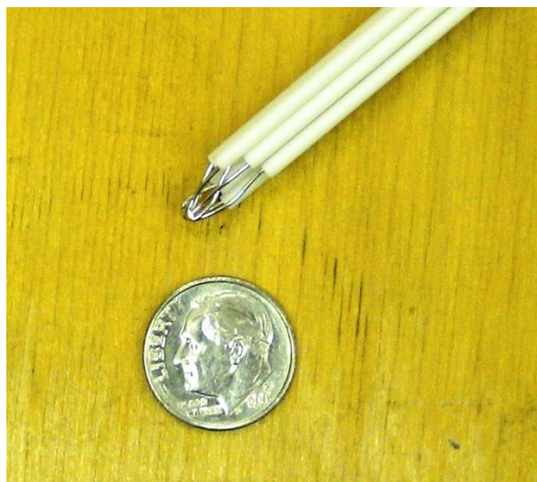
Fig. 1. Common measuring junction of the test bundle of eight platinum thermoelements as configured for use in the three-zone furnace tests.
