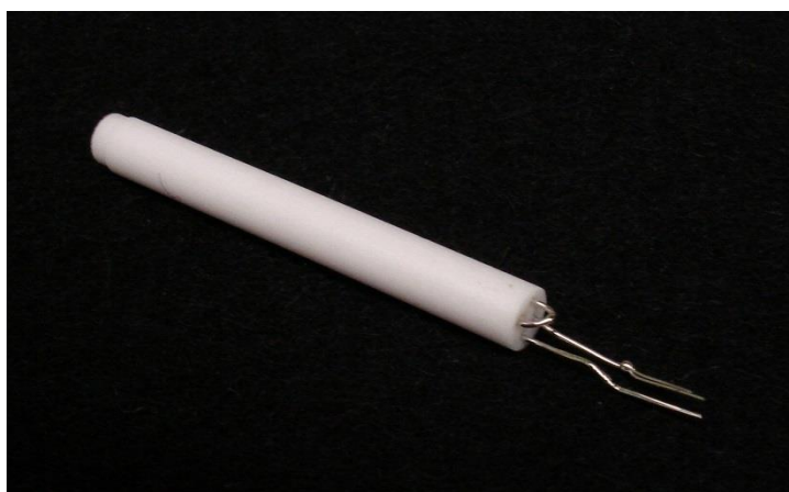
Figure 5. A completed resistor assembly from a 22 cm length of wire and a four-bore alumina insulator.
