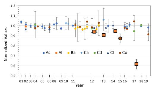
Figure 6. Stability of Selected Elements in SRM 1566b Oyster Tissue
