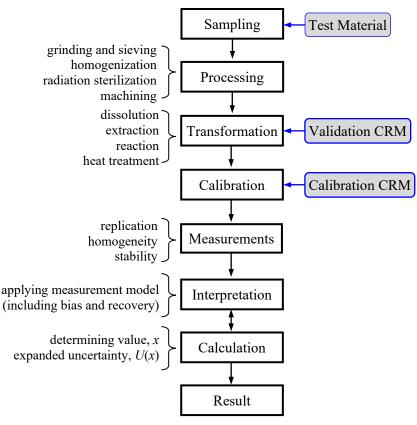
Figure 8. Steps in a Generic Measurement Process for Certifying Values
