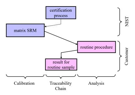
Figure 14. Metrological Traceability for Results When a Matrix Material is Used as a Calibrant
