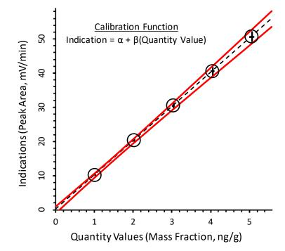
Figure 9. Quantity Values, Indications, and Calibration Function
