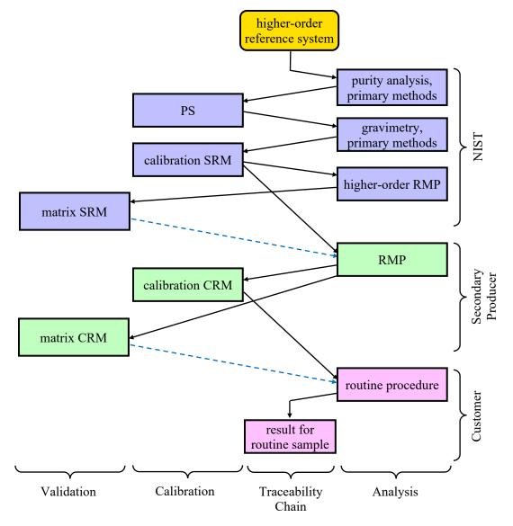
Figure 13. Metrological Traceability for Results Using NIST's Reference Materials
