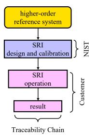
Figure 12. Metrological Traceability of Results from a NIST Standard Reference Instrument (SRI).
