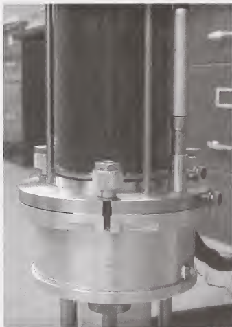
Figure 3. Tuning endplate assembly of cylindrical cavity.
