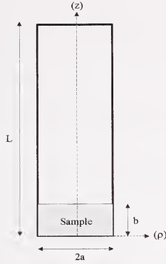
Figure 6. Sample-loaded circular-cylindrical cavity.
