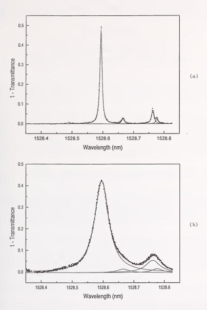
Figure 5. (a) Multiple line fit of line P6, low pressure cell. Of all the lines measured, P6 had the most significant contribution from nearby lines. (b) Multiple line fit of line P6, high pressure cell.
