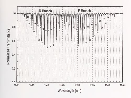
Figure 1. Acetylene  $(^{12}C_2H_2)$  spectrum taken by passing LED light through an absorption cell and recording the spectrum of the transmitted light using an optical spectrum analyzer with 0.05 nm resolution. This spectrum has been divided by the LED spectrum.
