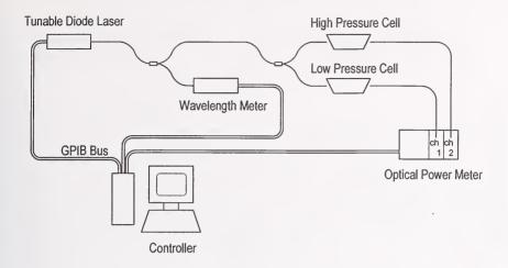
Figure 3. Schematic of the pressure-shift measurement apparatus.
