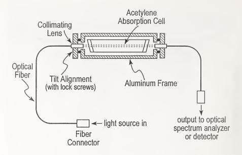
Figure 2. Schematic of fiber-pigtailed cell holder.
