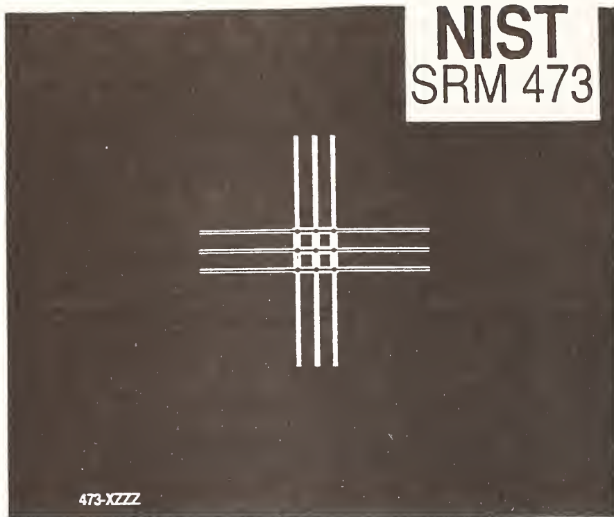
Figure 1. A view of the overall pattern on SRM 473. The basic measurement pattern is repeated eight times about the center. The horizontal and vertical lines help locate the patterns.
