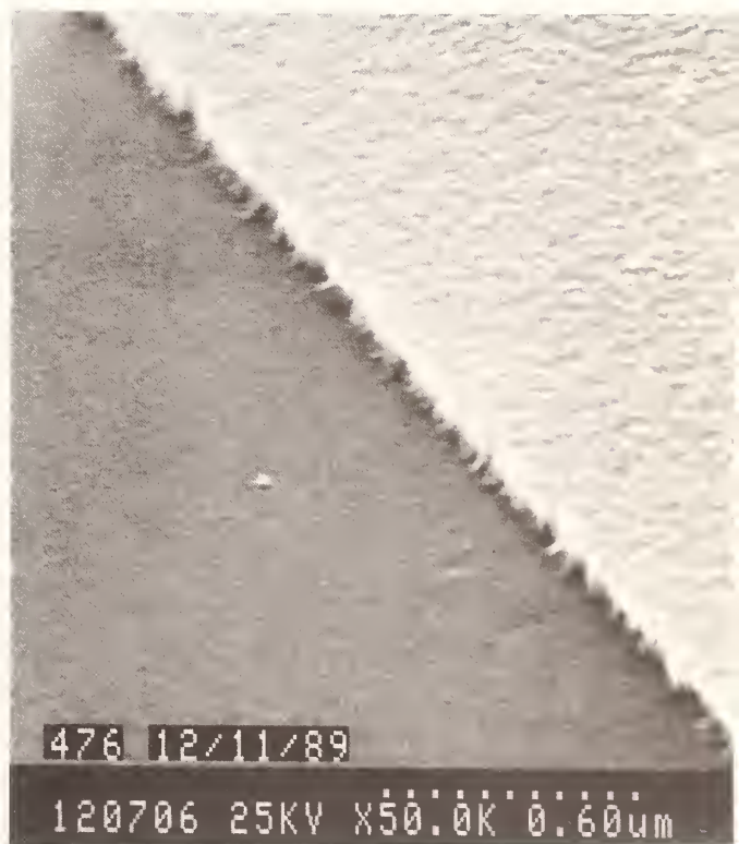
Figure 10. SEM photomicrographs showing the nonideal nature of line edges on a bright chromium photomask. The scale is indicated by the row of eleven dots in the lower right of each photomicrograph. In the upper photomicrograph, the dots are 0.03\ \mu\text{m} apart and in the lower photomicrograph, they are 0.06\ \mu\text{m} apart. Beam energy was 25 keV in both cases and the specimens were uncoated.
