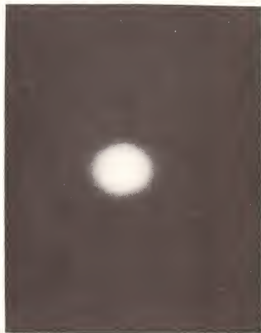
Figure 15. Normal and elongated 0.7- \mu\text{m} focal spots of 10- \mu\text{m} spheres.
