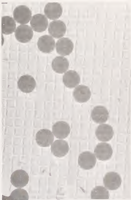
Figure 10—Electron micrograph of nominal one- \mu\text{m} polystyrene spheres (SRM 1690) at a magnification of 10,000\times . The spacing for the diffraction grating lines is 0.46 \mu\text{m} .
