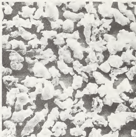
Figure 1. Scanning electron micrographs of the powders used to produce SRM 488. Mag. X160 a. as sized 310 stainless steel powder b. as sized 430 stainless steel powder
