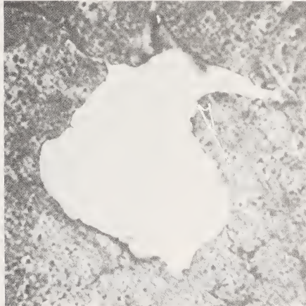
Figure 3. General microstructure of a compact. a. Optical micrograph showing the white austenite particles in the ferrite mixture. Mag. X50. b. Optical micrograph of an enlarged austenite particle. Mag. X800.
