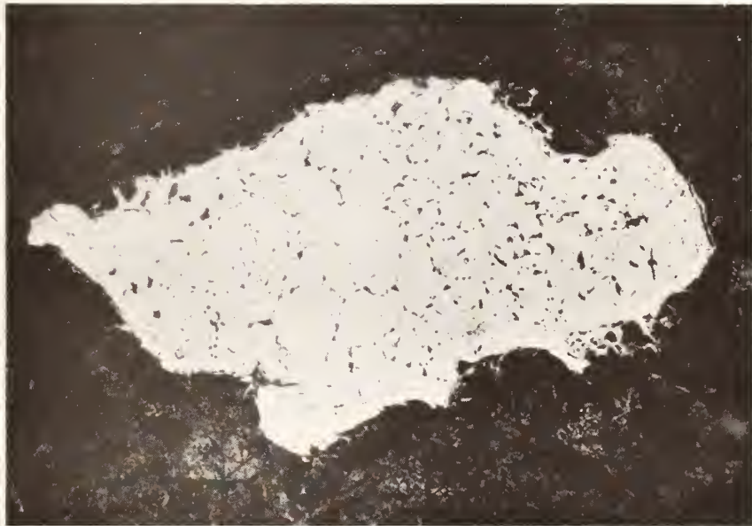
Figure 3. General Microstructure of a compact. a. Optical micrograph showing the white austenite particles in the ferrite mixture. Mag. X40. b. Optical micrograph of an enlarged austenite particle. Mag. X800.
