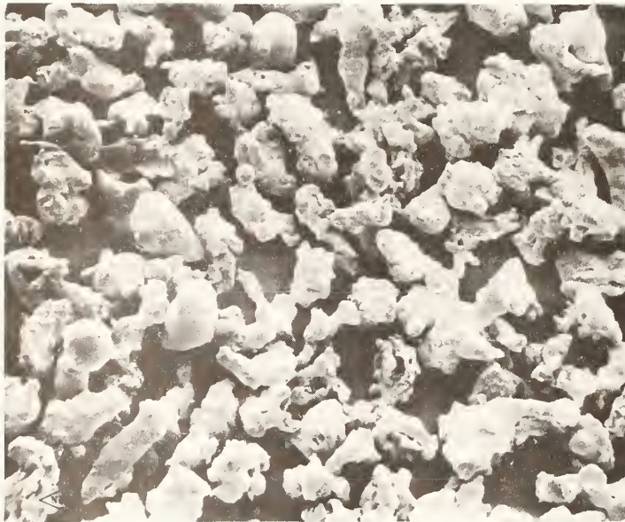
Figure 1. Scanning electron micrographs of the powders used to produce SRM 487. Mag. X160 a. as sized 310 stainless steel powder b. as sized 430 stainless steel powder
