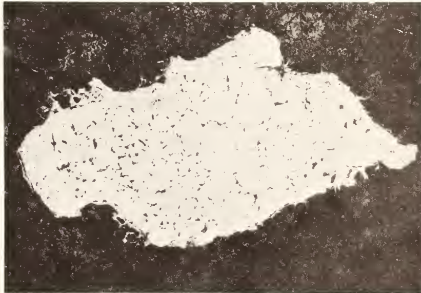
Figure 3. General microstructure of a compact. a. Optical micrograph showing the white austenite particles in the ferrite matrix. Magnification x40. b. Optical micrograph on an enlarged austenite particle. Magnification x800.
