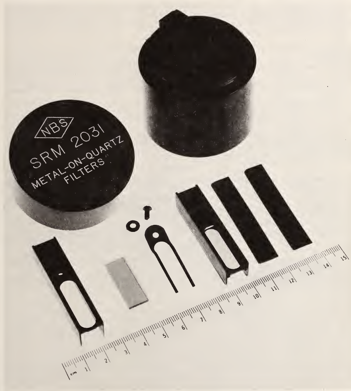
Top: Cylindrical container with its screw cap, both made of black-anodized aluminum alloy. Four filter holders can be stored in the cylindrical container. Bottom (from left to right): Aluminum alloy filter holder, 12.5 mm square and 58 mm high; Metal-on-quartz filter; Retaining spring of beryllium-copper with nylon screw and washer; Assembled unit; and Two Delrin shutters. All metal and plastic parts are flat black.
