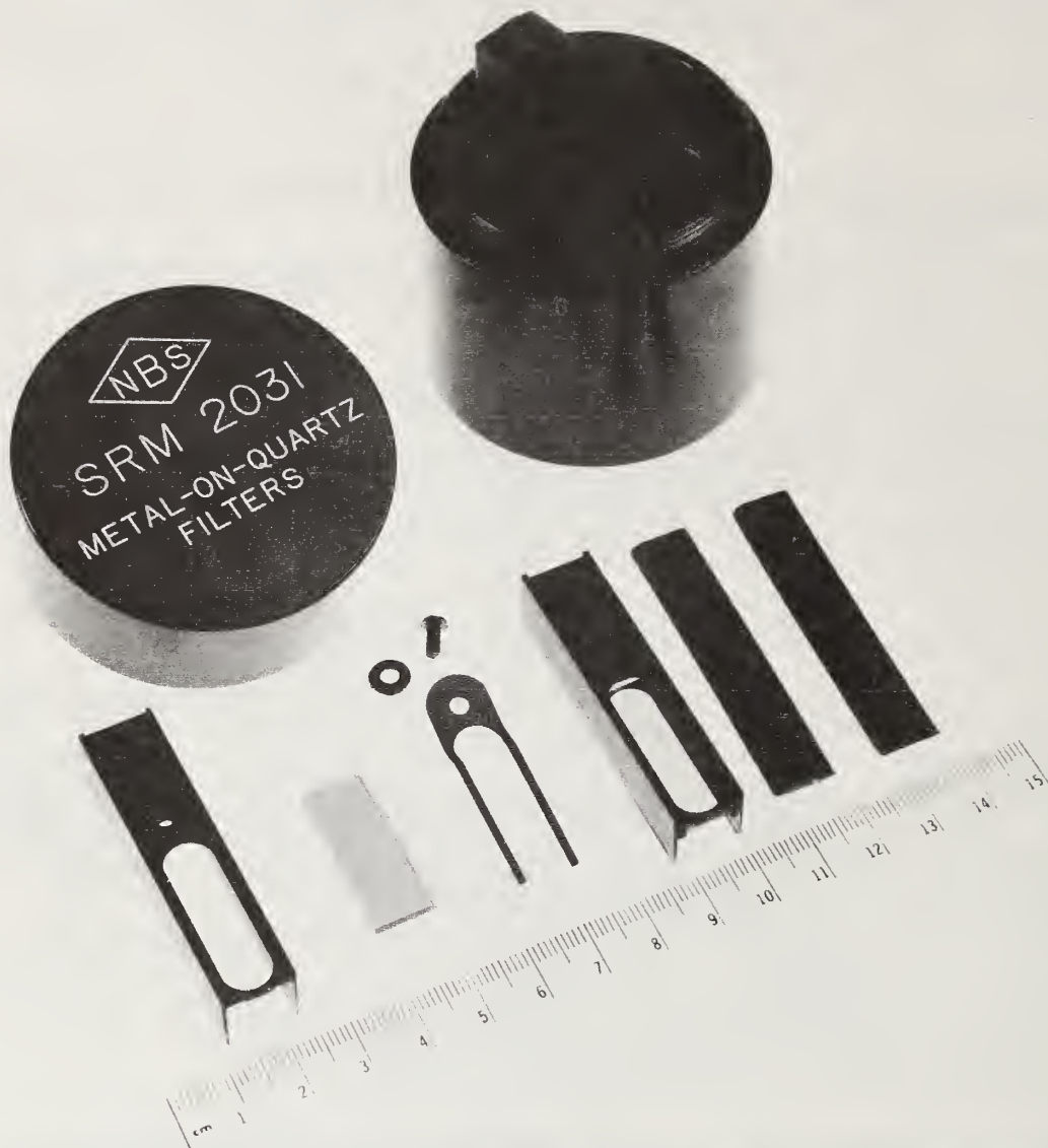
Figure 16. Illustration of SRM 2031, Metal-on-Quartz Filters for Spectrophotometry. This same figure illustrates the certificate for SRM 2031. See text for details.
