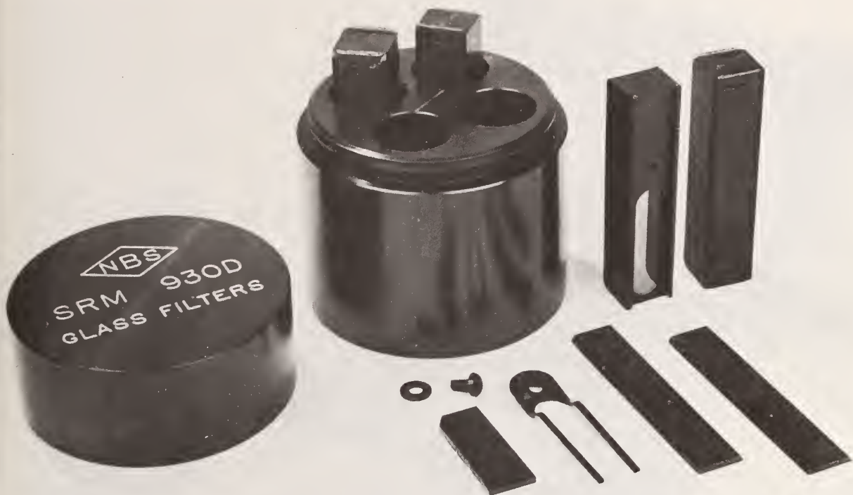
Figure 2. Illustration of SRM 930D, Glass Filters for Spectrophotometry, showing the black-anodized aluminum alloy container for storing three filters in their holders and an empty filter holder. One of the three glass filters, Schott NG4 and NG5, is shown with the retaining spring, nylon screw, washer, and the filter holder with the front and rear shutters.
