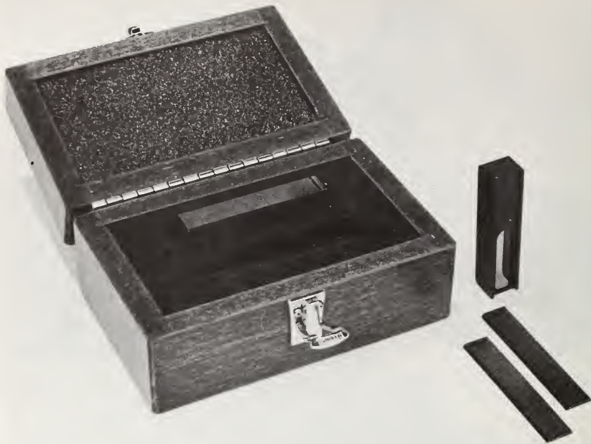
Figure 3. Illustration of SRM 2030, Glass Filter for Spectrophotometry, showing the glass filter, Schott NG4, in its metal holder with front and rear removable shutters. The wood-like plastic box is used to store the glass filter in its holder and an empty filter holder.
