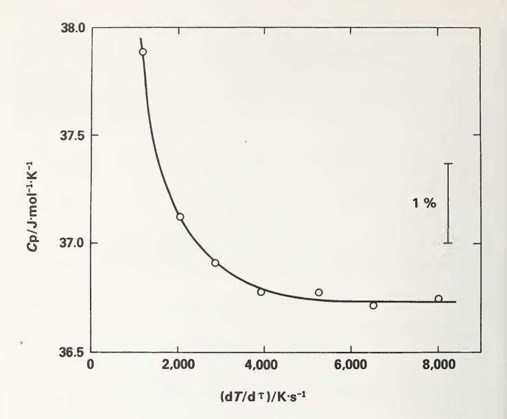
Figure 5. Dependence at 2000 K of calculated heat-capacity of SRM 781 molybdenum (specimen D2) on specimen-heating rate.
