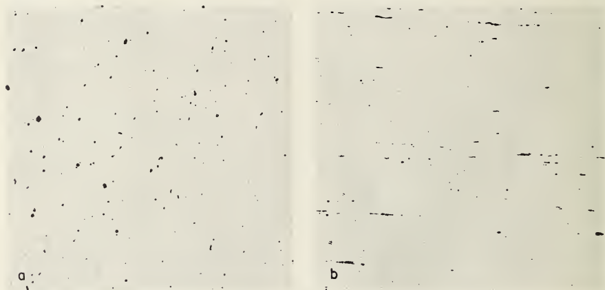
FIGURE 1. NBS 461 steel polished for inclusion counting and microprobe examination.
