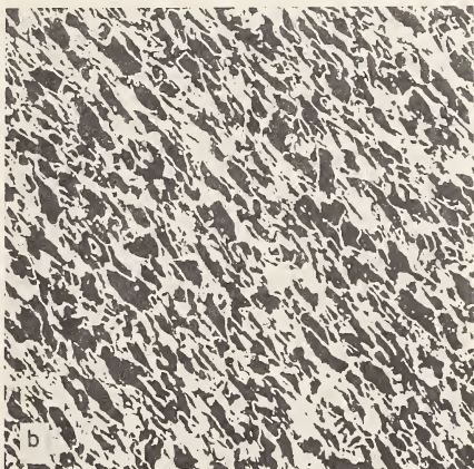
FIGURE 4. Longitudinal section of NBS 461 steel etched for 10 s in 3-1/2 percent \text{HNO}_3
