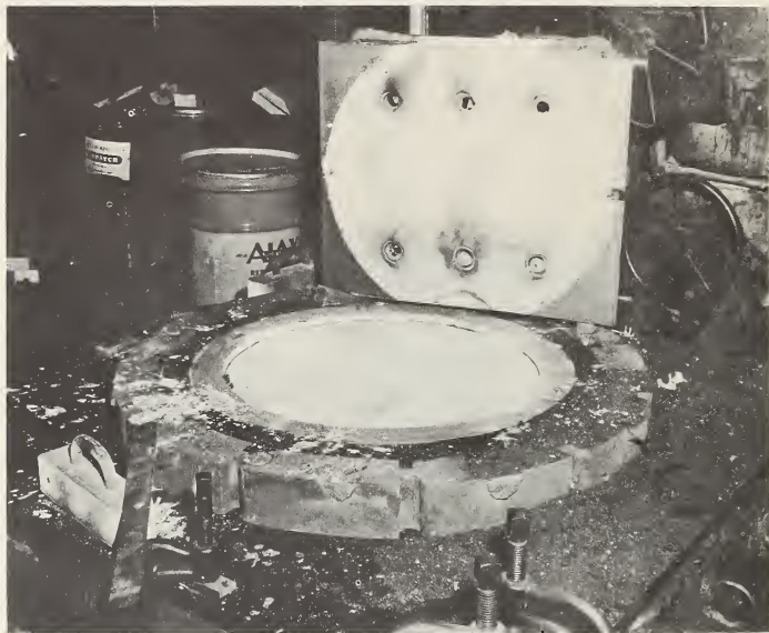
Figure 3. Solidified casting on the water-cooled copper plate after removal of pouring basin.
