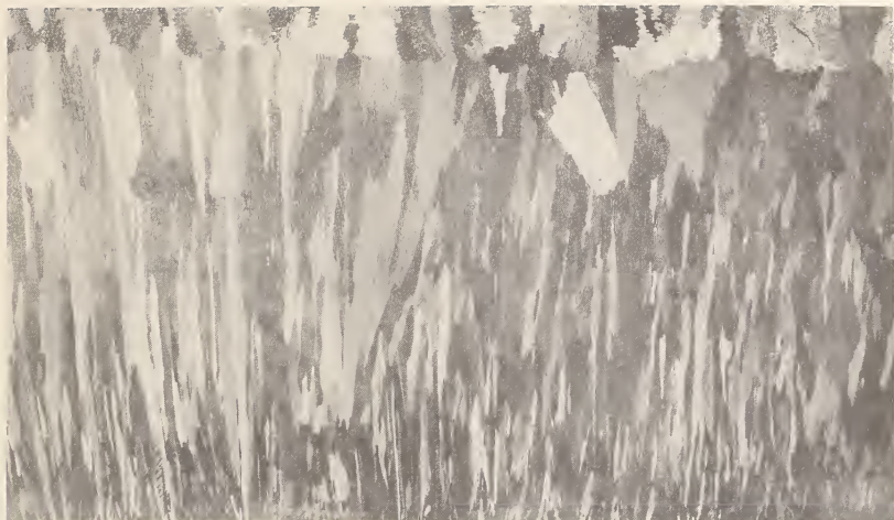
Figure 5. Typical etch pattern of the casting thickness.
