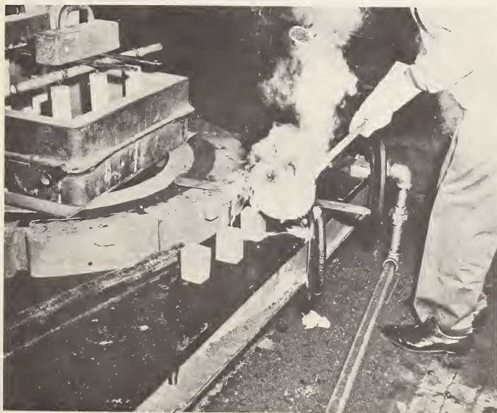
Figure 2. Pouring of test samples prior to pouring the molten metal into the stoppered pouring basin.
