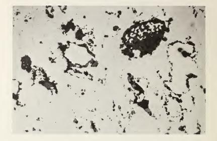
Figure 1. Final submitted stainless steel powder compact. Unetched X750.
