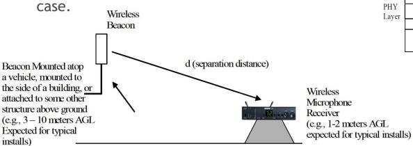
Figure B.1—Beacon/wireless system separation distance
