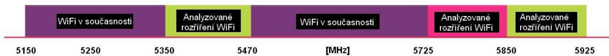
Figure No. 3 – Current and possible future configuration of the band of 5 GHz for FWA/WiFi
