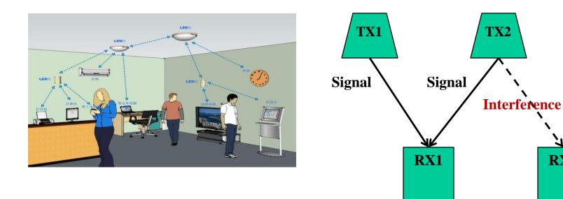
Multi-transmitter multi-receiver indoor visible light communication network
