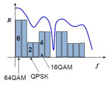
Closed-loop bit-/powerloading, bit-interleaved FEC, HARQ
