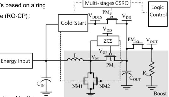
ZCS (Zero Current Switching) is designed for the efficient steady-state operation under ultra-low input voltages.
