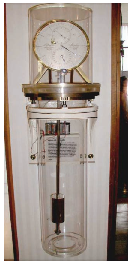
Figure 1. The Riefler pendulum clock, which was the primary standard for time interval measurements from 1904 to 1929, is now on display at the NIST museum in Gaithersburg, MD.
