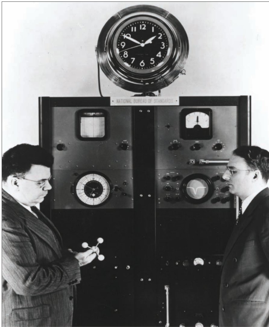
Figure 5. The first atomic frequency standard, based on the ammonia molecule (1949). Inventor Harold Lyons is on the right; Edward Condon, then the director of NBS, is on the left.
