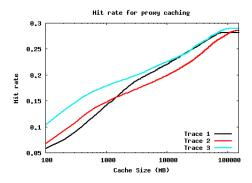
Figure 7. Hit rate based on proxy cache size
