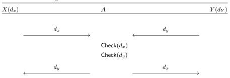
Fig. 1: Trivial FE protocol with a trusted third party arbitrator, A.
