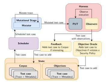
Figure 1: Fuzzer Architecture
