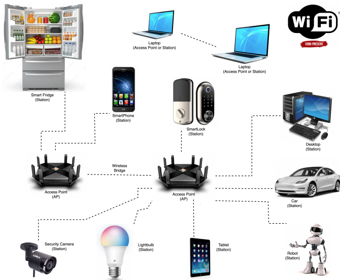
Fig. 1. Interconnection of Wi-Fi smart and AI devices.
