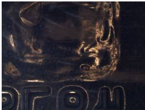
Fig. 2. Deformation due to heating of the forgery's backside.
