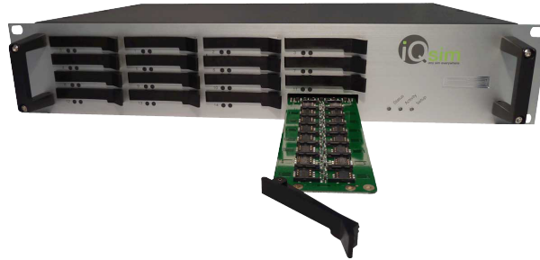
Fig. 21. An industrial multi-SIM reader.
