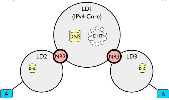
Core LDs maintain a database that contains the locators for each NID router connected to them. (It does <u>not</u> hold per-node state.)
