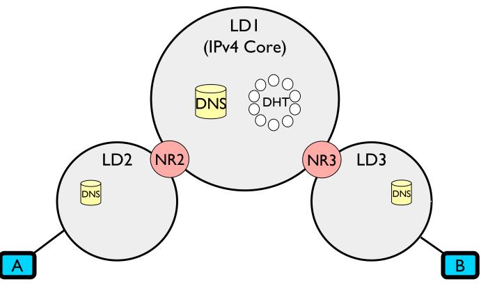
Domains are connected via NID Routers (NRs). These perform routing based on the destination NID, as well as locator mapping.
