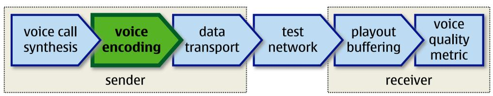
• sender encodes voice into audio frames for transmission across the network
