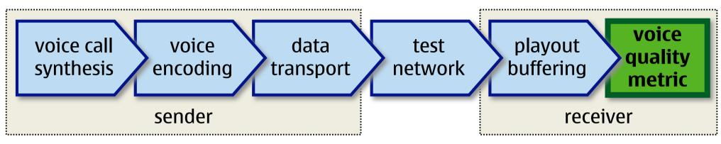
experiments use the ITU-T E-Model to compute the R-Score over a received audio frame sequence
