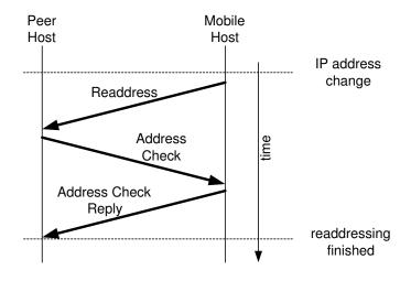
Figure 4.1: Packet flow for HIP readdressing
