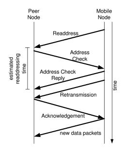
Figure 5.13: Packet flow after reconnection
