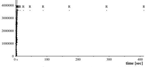
Figure 1.2: TCP retransmissions with exponential backoff
