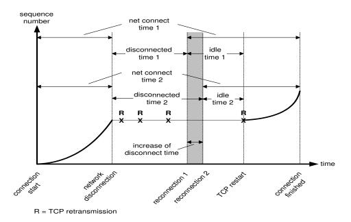
Figure 5.5: Idle time and net connect time with different disconnect times
