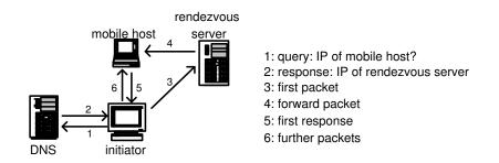
Figure 3.2: Initial communication setup using HIP
