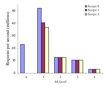
Figure 6.12. Mean aggregate lookup requests arriving at different levels of the AS hierarchy for different scopes.
