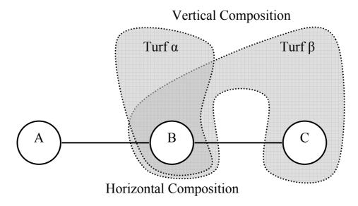
Figure 3.2. Vertical and horizontal composition of networks.
