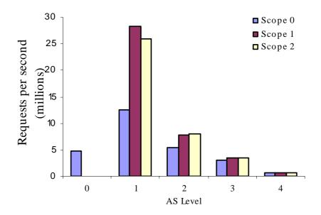
Figure 6.14. Mean aggregate lookup requests resolved at different levels of the AS hierarchy for different scopes.
