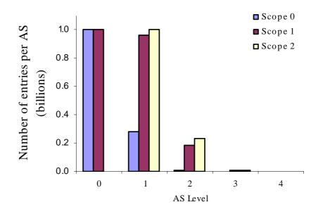
Figure 6.15. Mean registration table size per AS at different levels of the AS hierarchy for different scopes.
