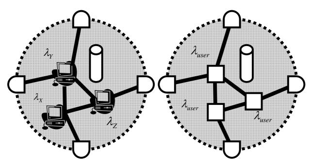
Figure 4.3. Equivalent model of the hosts and their communication rate.
