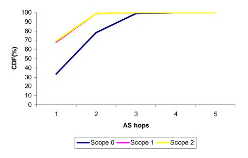
Figure 6.20. Cumulative Distribution Function of the AS hops until resolution depending on the scope.
