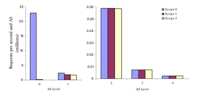
Figure 6.11. Mean lookup requests arriving at different levels of the AS hierarchy for different scopes.
