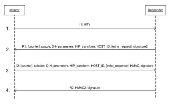
Figure 2.9: Host Identity Protocol Base Exchange.
