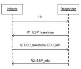
Figure 2.10: Setting up an ESP SA between HIP hosts during BEX
