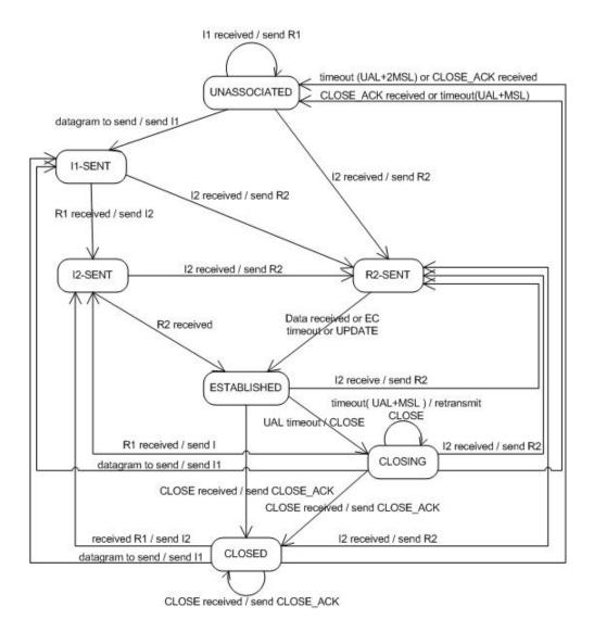
Figure 4.2: HIP state diagram
