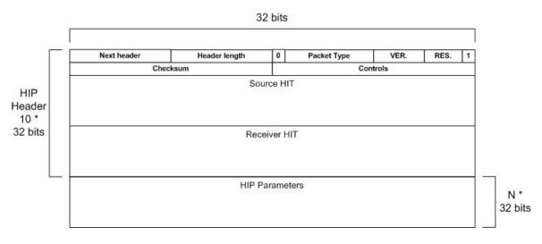
Figure 4.1: HIP PDU format.
