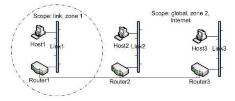
Figure 2.3: IPv6 address scopes.
