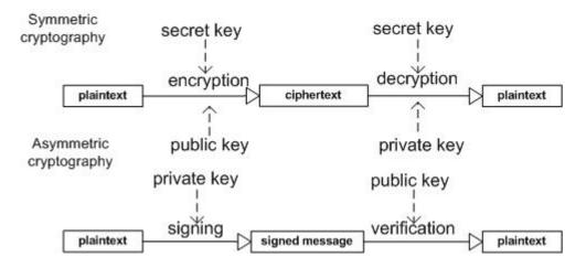
Figure 2.4: Symmetric and asymmetric cryptographical functions.
